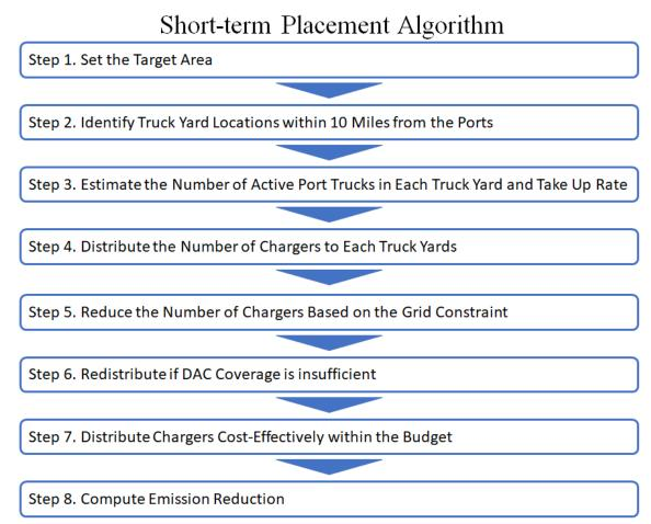
Figure 16. Overview of Short-term Placement Algorithm
